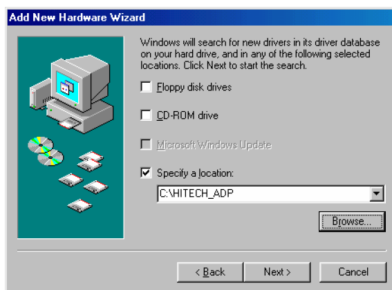
Figure D-19: Specify a the file directory where the device driver is stored. The default is C:\HITECH_ADP
