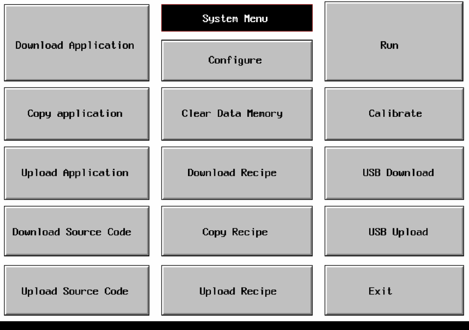
Download/Upload/Copy port: COM2 PLC communication port: COM2 Figure D-6: PWS3261 Calibrating Touch Panel
